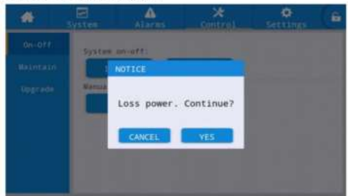
Fig. 4-6 Inverter shutdown pop-up window interface
